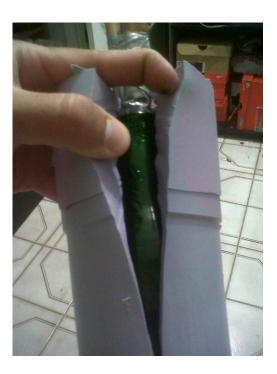
When the mold is cured cut down one side of the plastic bottle carefully because we are going to use that bottle later
