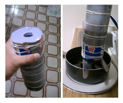
Pour the mix in the mold through the opening fill up at least half of the mold then rotate for 5 seconds and the turn upside down and let all the excess drip into the pot.
